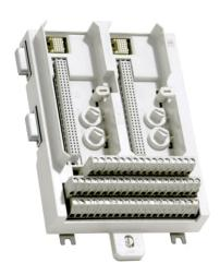
The TU842 MTU can have up to 16 I/O channels and 2+2 process voltage connections. Each channel has two I/O connections and one ZP connection. The maximum rated voltage is 50 V and maximum rated current is 3 A per channel.
