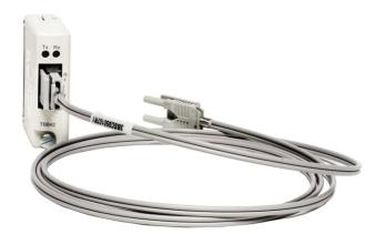
TB842 ModuleBus Optical Port is a communication interface between the Cl801 or Cl840/Cl840A FCI and the TB820/TB820V2/TB840/TB840A ModuleBus modem of an I/O cluster or ABB drives units via the Optical ModuleBus. TB842 connects to Cl801 via TB806 and to Cl840/Cl840A via TU847 and TB806 for single I/O or via TU846 and TB846 for redundant I/O.
