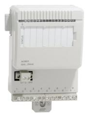
The AO801 Analog Output Module has 8 unipolar analog output channels. The module performs selfdiagnostic cyclically. A low internal power supply sets the module in INIT state (no signal from the module).
