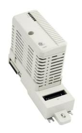
S100 I/O communication is realized in AC 800M by communication interface CI856, which is connected to the CEX-Bus through a base plate. The baseplate, TP856, houses a ribbon connector connecting to bus extender boards in S100 I/O racks and provides a simple DIN-rail mounting. Up to five S100 I/O racks can be connected to one CI856 where each I/O rack can hold up to 20 I/O boards.
