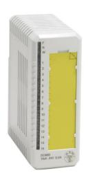
The DO880 is a 16 channel 24 V digital output module for single or redundant application. The maximum continuous output current per channel is 0.5 A. The outputs are current limited and protected against over temperature. Each output channel consists of a current limited and over temperature protected high side driver, EMC protection components, inductive load suppression, output state indication LED and an isolation barrier to the Modulebus.
