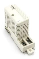
PROFIBUS DP is a high speed multipurpose bus protocol (up to 12Mbit/s) for interconnecting field devices, like remote I/O, drives, low voltage electrical equipment, and controllers. PROFIBUS DP can be connected to the AC 800M via the CI854B communication interface. The CI854B includes two PROFIBUS ports to realize line redundancy and it also supports PROFIBUS master redundancy.
